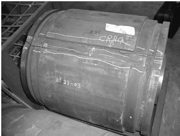
Figure 4. A container that has been overheated
