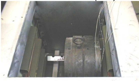
Figure 1. Die oven development, showing an instrumented die being monitored to ensure that overheating cannot occur in service
